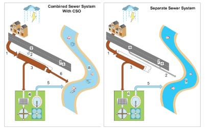
Figure 1: Combined and separate sewer system.
