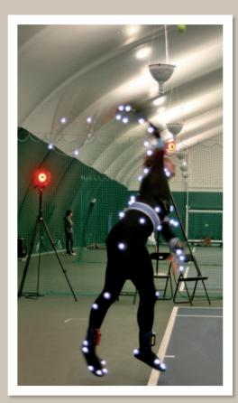
The small stable sensors worn by this tennis player provide researchers from the CLARITY Centre for Senor Web Technologies with data on the athlete's movement. The team is working on a wearable sensor system that provides feedback on sporting and rehabilitation movements, which may help people heal faster from injury, perform better in sports and live healthier lives. The photo, taken by Matthew Patterson UCD School of Physiotherapy & Performance Science, is shot in Dublin City Univeristy.
